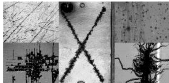
Figure 4. Various Surface Defects for Binary Image Analysis
