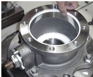
Figure 16 - Body Seal Installation
