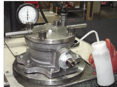
Figure 14 - Valve Stem Leak Test
