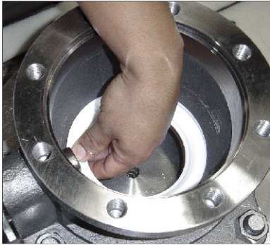
Figure 15 - Installing First Ball Seal
