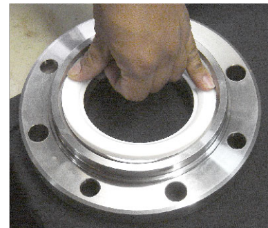
Figure 19 - Installing Ball Seal in Cap Plate
