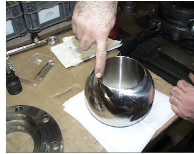
Figure 17 - Checking for Nicks
