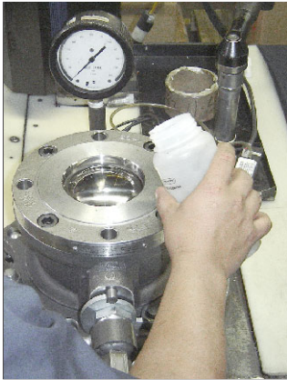
Figure 25 - Immersing Seal for Leak Test
