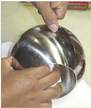
Figure 7 - Checking Scratch Severity
