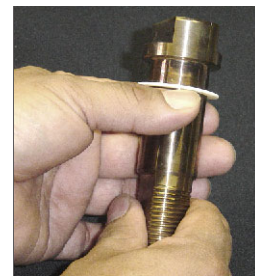
Figure 10 - Installing Thrust Washer
