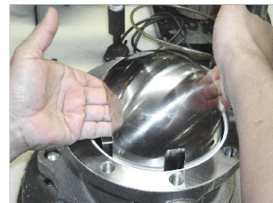
Figure 18 - Placing the Valve Ball
